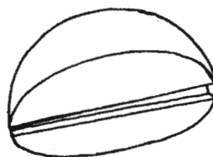
Figure 12 Lead bar shot half (no. 33605). The central groove in the face will be noticed. The other half would also have this groove. When put together, the central groove in the combined halves would be
